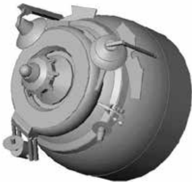
Figure 31 Spacecraft geometry with superstructures. Pressure gauges P1 and P2 are located and seen on the right side of the surface.
