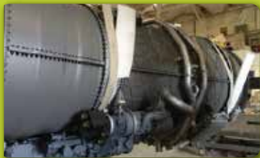
Pratt Whitney F135 full-scale engine mock-up used to validate fit and clearance. Majority parts produced on Stratasys FDM machines.
