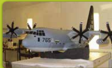
Model of Lockheed Martin C-130. The scoops on its wings and details on fuselage comprised of 3D printed parts.
