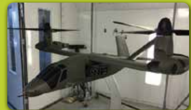
Model of Bell AV280. All fairings, weapons, and blisters on the fuselage were created with Stratasys 3D printers.
