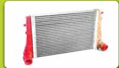
FDS Intercooler with 3D printed end tanks for live testing with thermocouples. (The right side of the tank is strengthened for extreme temperatures.)
