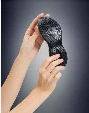
Flexible shoe sole produced on the Objet30 Prime 3D Printer
